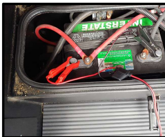
RV HOUSE BATTERY, W/ CHARGE CLAMPS
