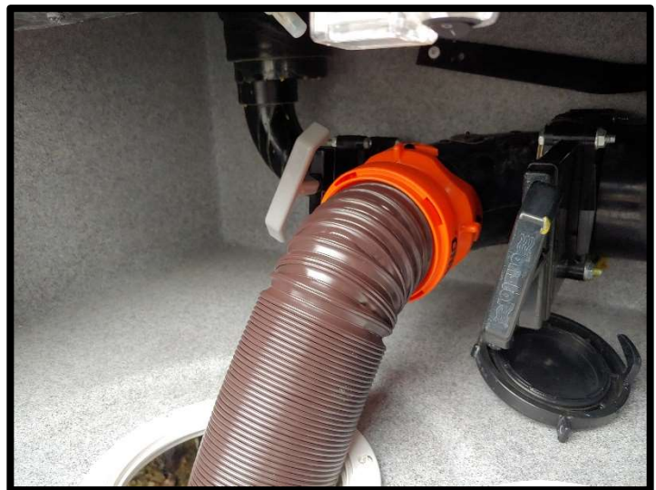
RUN WASTE HOSE INTO COMPARTMENT, ATTACH TO DRAIN
